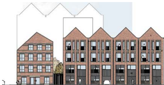
Proposed George Leigh St elevation incorporating the retained building on the left
